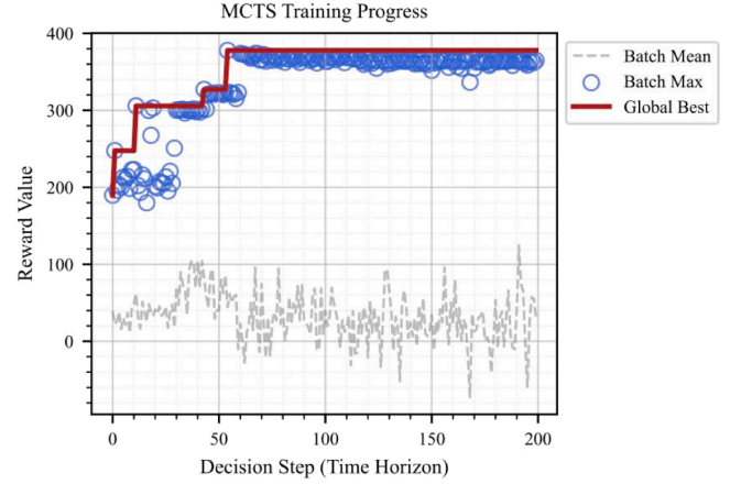
Fig. 18. Diagram of the learning curve of the MCTS method in 5-stage strict multistage collision scenario.
